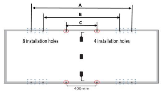
$\diamond$  Use mounting holes of A or B or C , safety factor  $\gamma_{m=1,5}$ , and this value can decrease if modules are not mounted following the instructions above.
